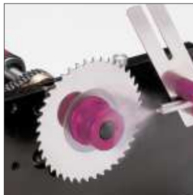
The micro-fine spray mist adheres securely to the saw blade, even at high speed.
