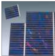
Machining Si-solar elements with a cut width of 0.2 mm.
