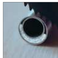
Cutting a V2A double pipe with fibre optic light guides for the endoscopy.
