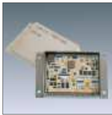
Opening a high-grade hybrid module for repair purposes.
