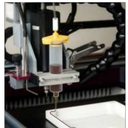
The cartridge is positioned in front of the milling cutter by a clamping adapter.
